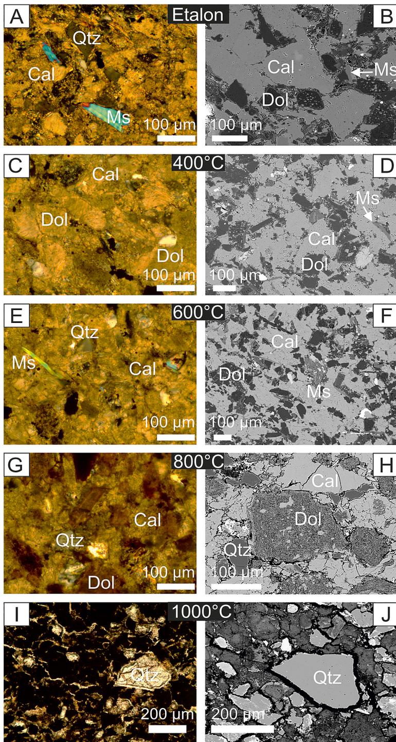
Fig. 6. Spišské Tomášovce sandstone microstructural changes after the heating visualized in polarizing microscope (left column) and BSE (right column).
