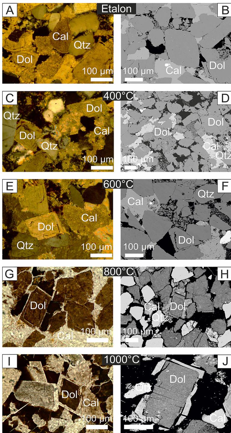
Fig. 5. Králiky sandstone microstructural changes caused by heating observed in polarizing microscope (left column) versus BSE (right column). Used abbreviations: Qtz - quartz, Dol - dolomite, Cal - calcite, BSE - back scattered electron.
