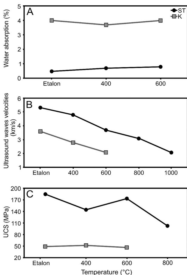
**Fig. 9.** Temperature versus physical properties of the sandstones: A – water absorption; B – ultrasound wave velocities; C – uniaxial compressive strength.
