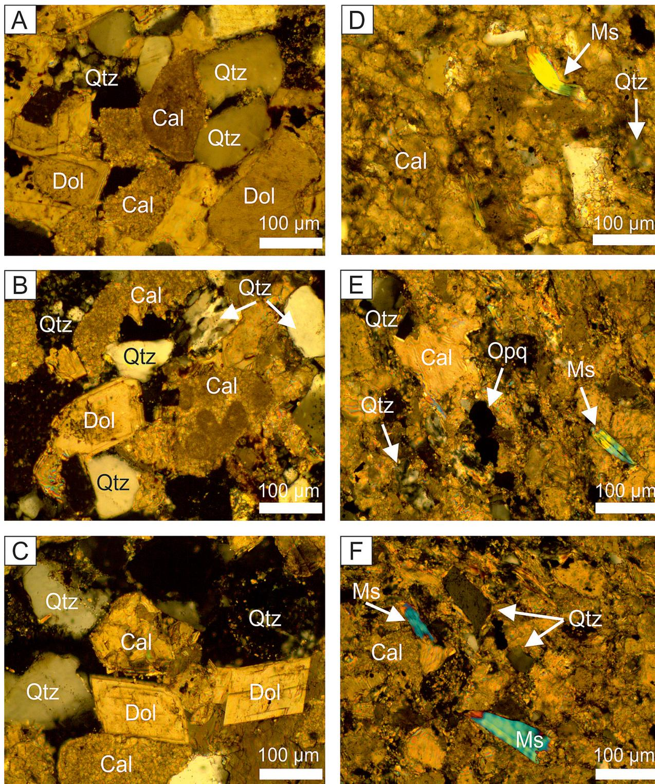
Fig. 4. Microstructure comparison of etalon sample sandstones in cross polarized light: Králiky sandstone (A, B, C); Spišské Tomášovce sandstone (D, E, F).
