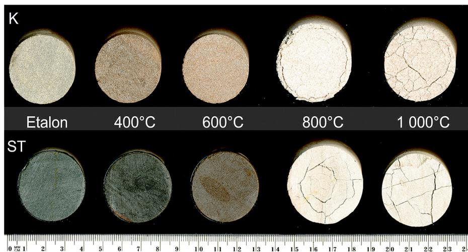
Fig. 2. Tested sandstones and temperature to which they were exposed: K – Králiky, ST – Spišské Tomášovce.
