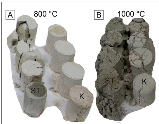
Fig. 3. The disintegration of sandstones after the heating at: A – 800 °C; B – 1000 °C. K – Králiky, ST – Spišské Tomášovce.
