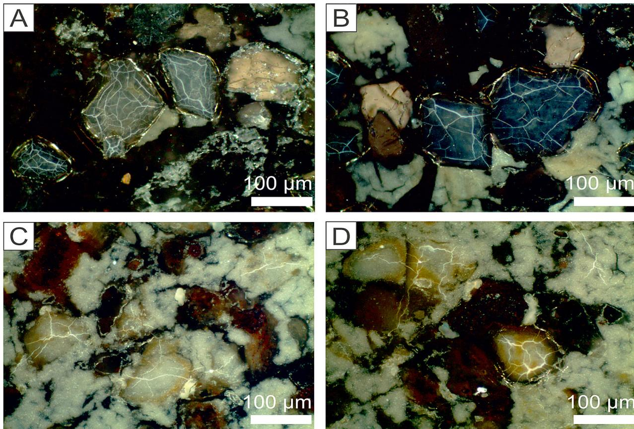
Fig. 7. Creation of micro-cracks in quartz grains of sandstones after their heating at 1000 °C: A–B) Králiky; C–D) Spišské Tomášovce.
