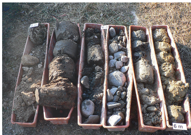
Fig. 3: Heterogeneous material in the core sample of well 3. Photo: D. Krčmář
