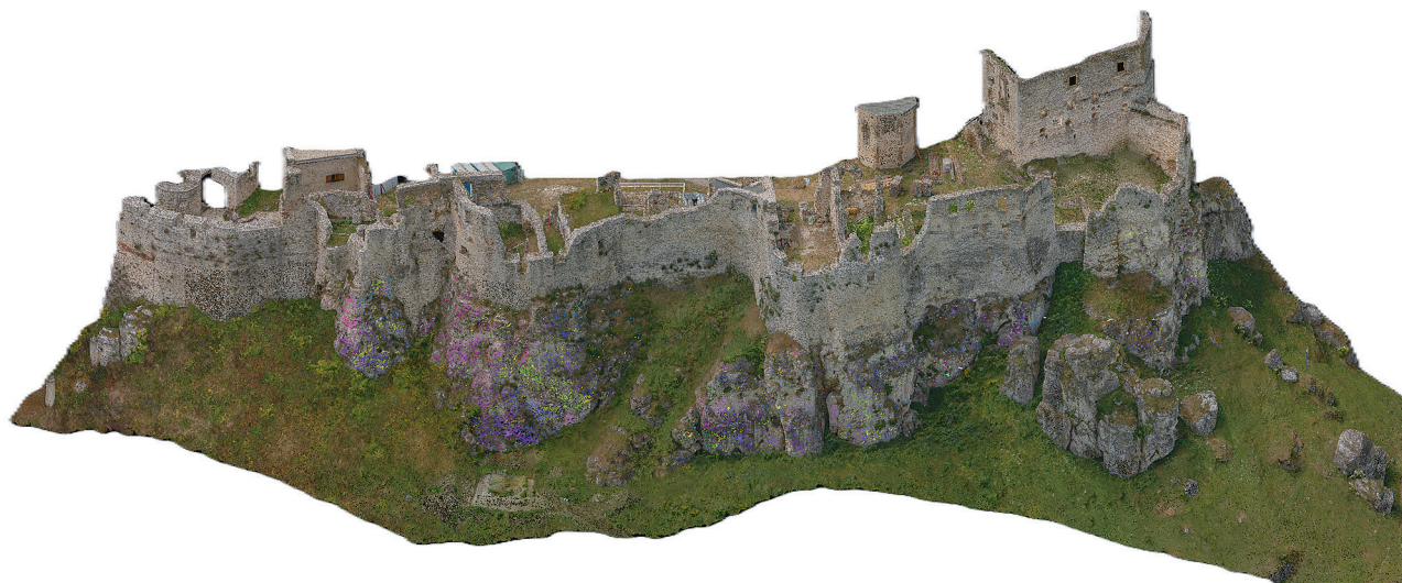
Fig.2. The following visual representation illustrates the 3D point cloud, showcasing the rock slopes situated at the base of the eastern palaces within the surveyed section of Spiš Castle. Discontinuities in the rock massif are marked in color.
