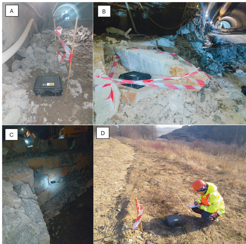
Fig. 5: Position of seismographs at the site Homole tunnel (A: in tunnel; B: on the portal; C: on the tunnel stage; D: on the ground directly above the blast)
