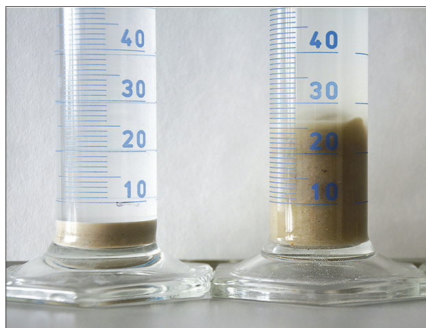
Fig. 1. Example of swelling bentonites after Swell index test (ASTM D5890). ELU at 25 °C left and RLU at 25 °C right.
