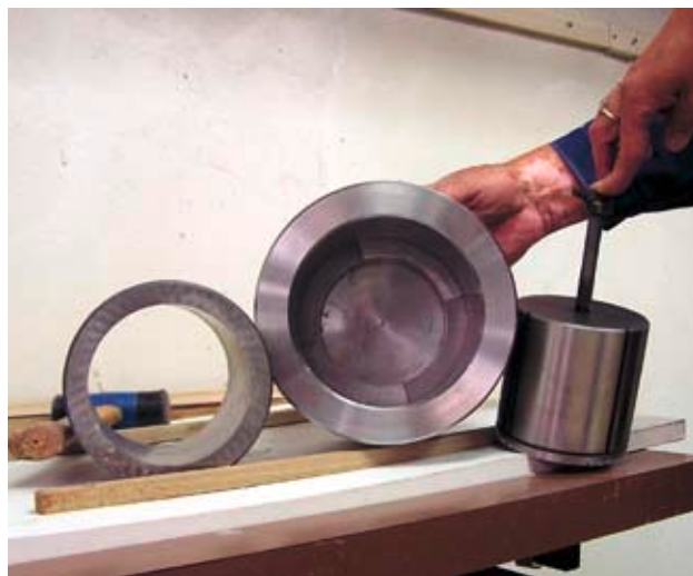
Fig. 4. Second compaction mould – for \varnothing 100 mm bentonite cylinders.
