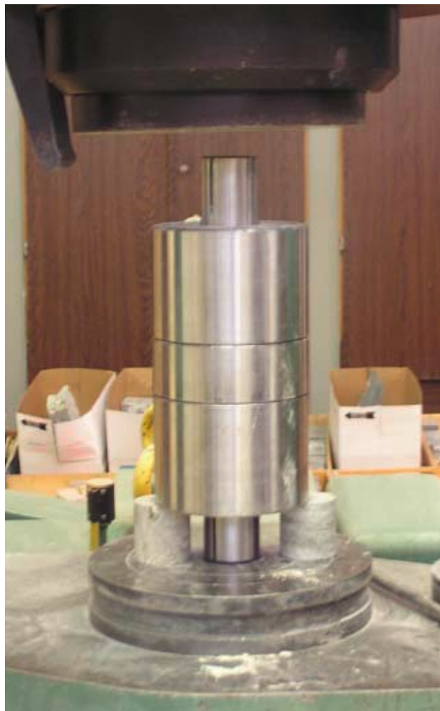
Fig. 3. First compaction mould prepared to press \varnothing 50 mm bentonite cylinders.
