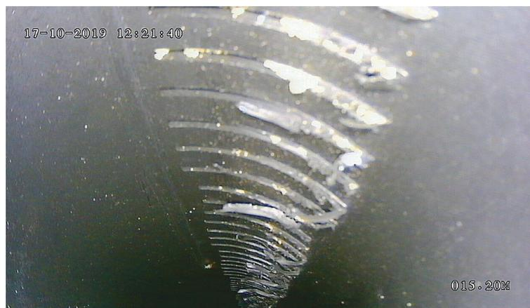
Fig. 5.: View from a camera record of a horizontal drainage borehole – without colmatation.
