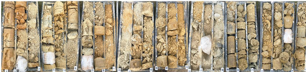
Fig. 4.: Cores of the borehole MI-INK-1, MI-INK-2 and MI-INK-4 in the order as they are located on the interpreted profile
