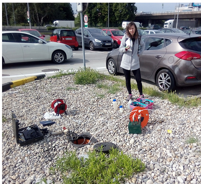
Fig. 7. Groundwater sampling and recording of data from data loggers on groundwater temperature and table level in well A-3
