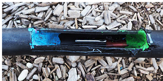
Fig. 6. PT100 thermistor port for temperature measurement (Křmář et al., 2019)
