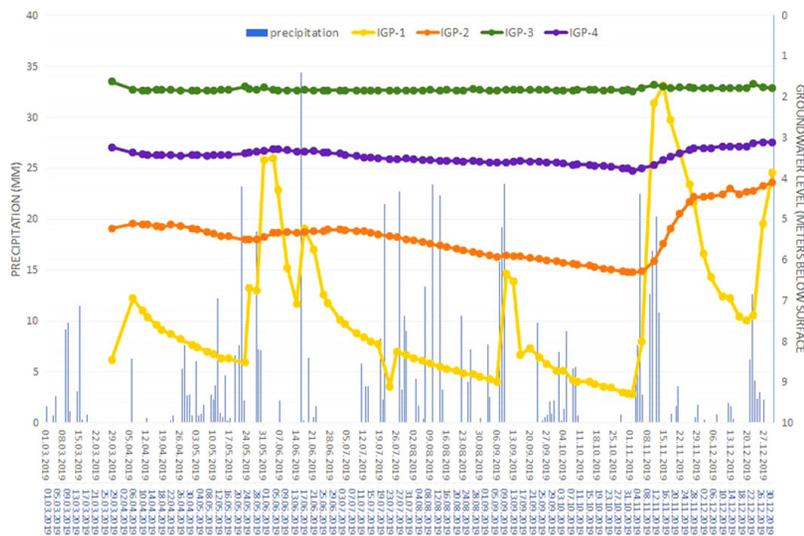
**Fig. 5.** Graph demonstrating groundwater level oscillations in boreholes and daily precipitation amounts from March to December 2019 (groundwater level observations: author’s data; precipitation amounts: SHMÚ (Slovak Hydrometeorological Institute).
