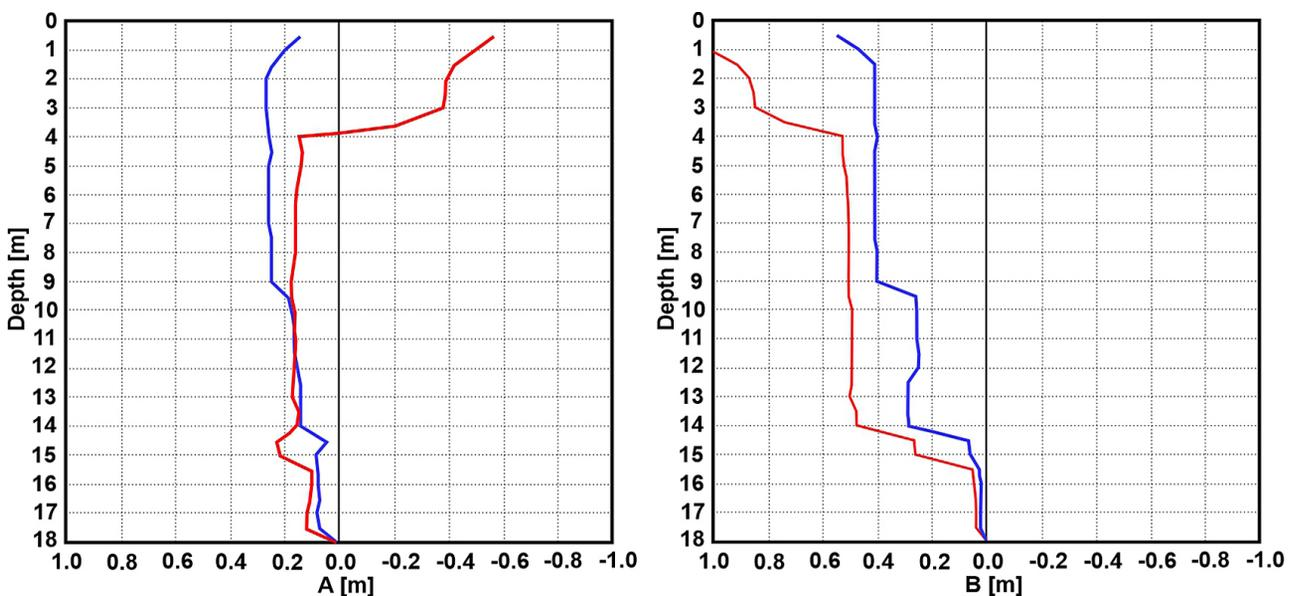
Fig. 7. An example of processed inclinometer measurement; borehole IGI-1, vertical black line- zero measurement, blue curve- first measurement, red curve- second measurement; direction A – left, direction B – right.
