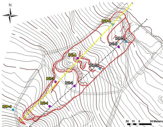
Fig. 4. Map of landslide with boreholes' location: blue - piezometric boreholes, violet - inclinometer boreholes; a profile chosen for stability calculations – yellow line using boreholes' documentation from yellow signed boreholes (modified according to Tupý et al., 2019).
