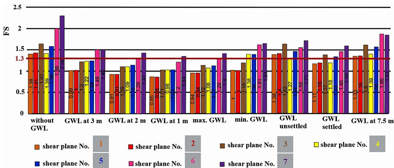
Fig. 9. Graphical expression of FS values calculated for 7 different shear planes at different groundwater levels.
