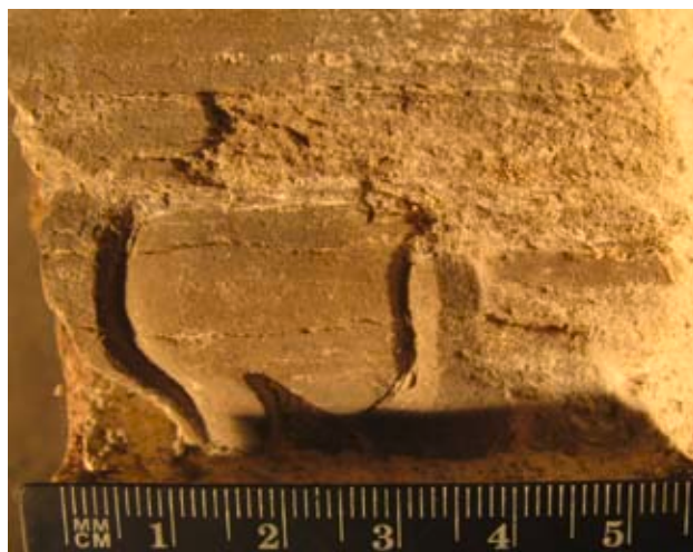
Fig. 8. Yellowish sandstone from the tabernacle of the St. Emmeram's Cathedral is crinoidal limestone (sandstone), Tata Limestone Fm. which was formed in middle part of the Cretaceous. It comes most probably from the northern Hungary.
