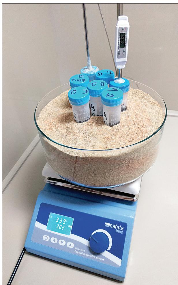
**Fig. 1.** Experimental setup of leaching of the authigenic phase from powdered clay sediment. Each sample tube contains 1.5 g of powdered sediment, 30 ml of leaching solution and a stirring magnet.
