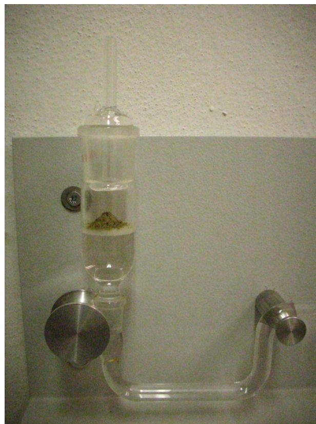
Fig. 10. Enslin-Neff test. Conus of the rock powder in the center of the water-saturated porous plate enabling suction and absorption of water.
