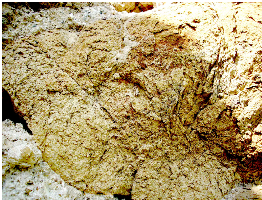
Fig. 5. Highly altered building stone: yellowish color, disintegration into small grains along many fine cracks. Length of the block ca. 500 mm.
