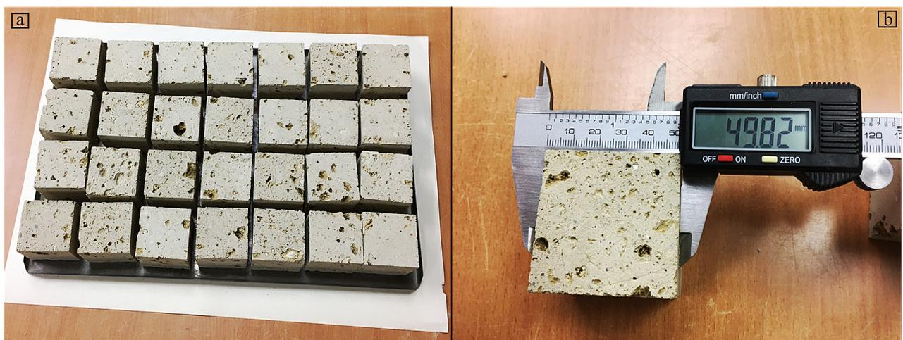
**Fig. 3:** Tuff samples. a – one part of the tuff cubes prepared for the application of the protective coating; b – a more detailed view of the tuff showing the remarkable macro-porosity.
