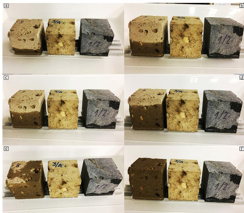
**Fig. 8:** Progress of the water absorption by capillarity over time is evident from the colour change of the saturated part in the yellowish tuff samples (compared to a grey low-porosity andesite as a contrast). a – after 10 minutes, b – after 30 minutes, c – after 60 minutes, d – after 2 hours, e – after 3 hours, f – after 4 hours. Explanatory notes: the first cube from left to right is an untreated sample in all photos; the second one is the sample coated by Antipluviol S.
