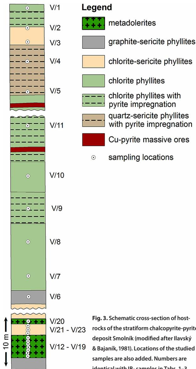
Fig. 3. Schematic cross-section of host-rocks of the stratiform chalcopyrite-pyrite deposit Smolník (modified after Ilavský & Bajaník, 1981). Locations of the studied samples are also added. Numbers are identical with IB-samples in Tabs. 1-3.
