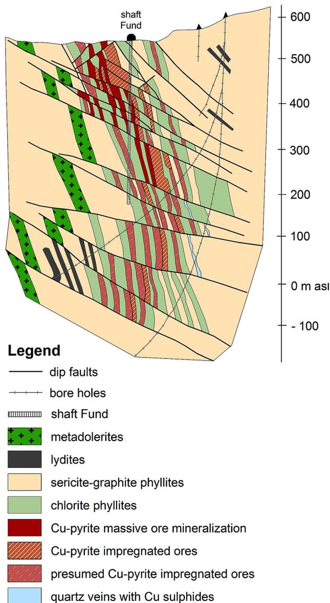
Fig. 2. Schematic section of the stratiform chalcopyrite-pyrite deposit of Smolník (modified after Ilavský, 1964)
