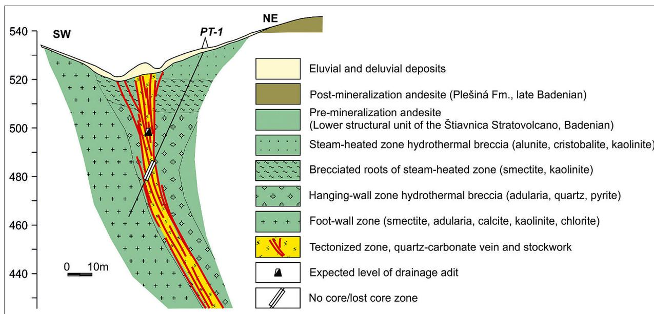
**Fig. 4.** Schematic cross-section along the PT-1 drill hole at the Prochot-Lazy site with interpreted position of mineralised vein structure and individual alteration zones.
