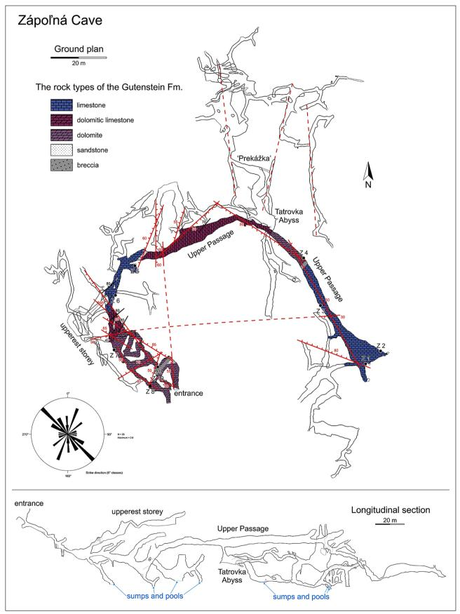
Fig. 3. Ground plan and longitudinal profile of the Zápoľná Cave. The ground plan contains mapped rock types, marked places of sample collection (black dots from Z-1 to Z-10), orientation of the bedding planes (black lines), mapped (ticked lines) and expected (dashed lines) faults. The orientation of discontinuities measured in the Zápoľná Cave is shown in the rose diagram created by Stereo32 software (Röller & Trepmann, 2003).
