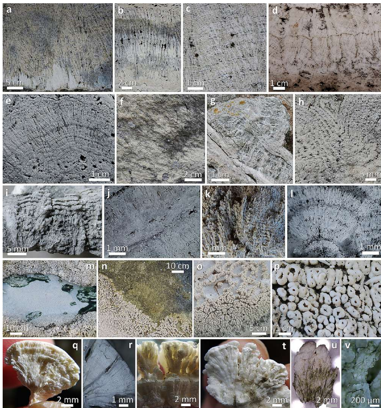
Appendix 3. Fan-laminated and dendrite-laminated crystals. a – fan-laminated crystals superposed shrub-crystals in Spiš travertine, b – fan-laminated crystals superposed dendrite crystals in Spiš travertine, c – fan-laminated crystals in Spiš travertine, d – fan crystals with indistinct laminae in Spiš travertine, e – dendrite-laminated crystals in Spiš travertine, f – fan-laminated crystals with distinct wavy lamination and invisible to the naked eye dendrite crystals in Ostrá hora (original dip), g – fan-laminated crystals in possible spelethems in Spiš castle, i – shrub crystals passed to fan-laminated crystals in Levice Vápnik, j – fan-laminated crystals in Hranovnica Malacinová, k – dendrite-laminated crystals in Dreveník quarry, l – fan-laminated crystals in Ostrá hora, and m–v – tooth-like shrubs with fan-laminated and dendrite-laminated crystals ( m – shrubs along a channel in Dudince, n–o – shrub clusters with and without cyanobacterial growth in Santovka, p – tooth-like shrubs in Dudince, q–r – fan-laminated crystals in Santovka, s–t – dendrite-laminated crystals influenced by cyanobacteria in Santovka, u–v – mineral habit influenced by cyanobacteria filaments in Santovka).
