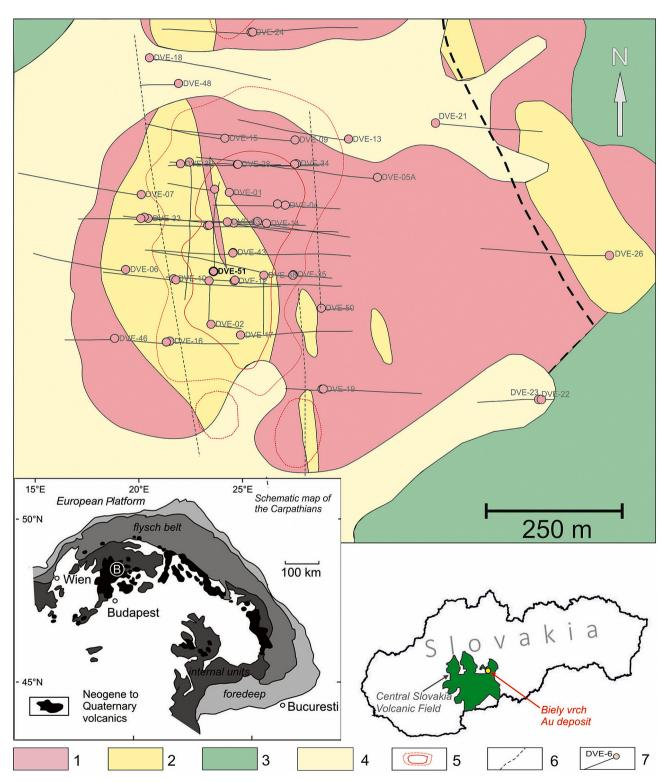
Fig. 2. Geology of studied area with drillhole plan. Legend: 1 – diorite porphyry; 2 – advanced argillic alteration zones of the diorite porphyry; 3 – andesite of the Stará Huta Formation; 4 – alluvial and deluvial deposits; 5 – quartz stockwork; 6 – faults; 7 – drill holes collar and drill hole lines.
