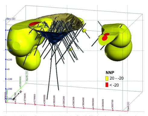
Fig. 6. 3D model (in coordinate system UTM-34U/ WGS84 ellipsoid) of the planned quarry and its surrounding, showing the parts with NNP in the area of uncertainty (yellow colour, in the range from -20 to 20) and parts in the area of potential acidity formation (red colour, below -20). Note: shades of yellow colour represented shading to highlight the 3D effect.
