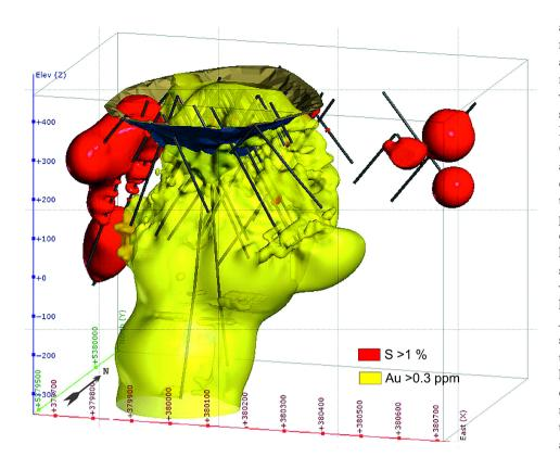
**Fig. 5.** 3D model (in coordinate system UTM-34U/WGS84 ellipsoid) of the planned quarry and its surrounding, showing the parts with sulphur content over 1% and Au content over 0.3 mg.kg<sup>-1</sup>. Note: shades of yellow colour represented shading to highlight the 3D effect.
