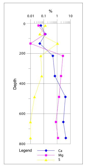
Fig. 4. Total content of Ca, Mg and S in the profile of the borehole DVE-51.
