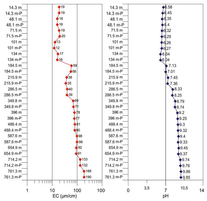
Fig. 3. The pH values and conductivity in the profile of the borehole DVE-51 (measured in water leachate).
