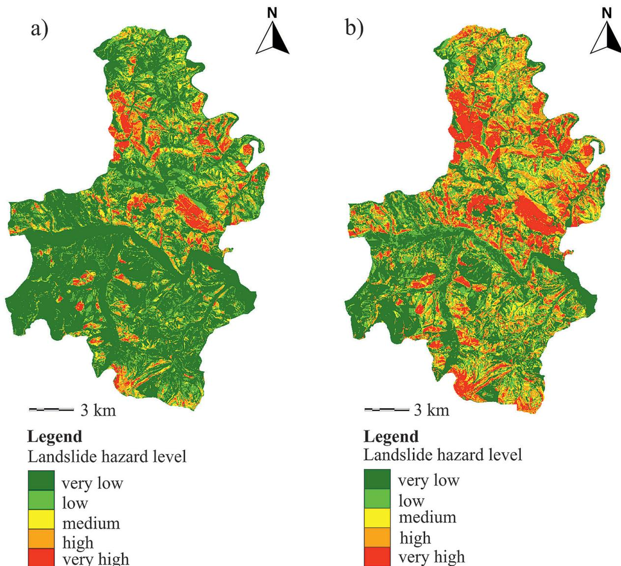
Fig 3. LSMs for the selected region (a–natural breaks; b–quantile)
