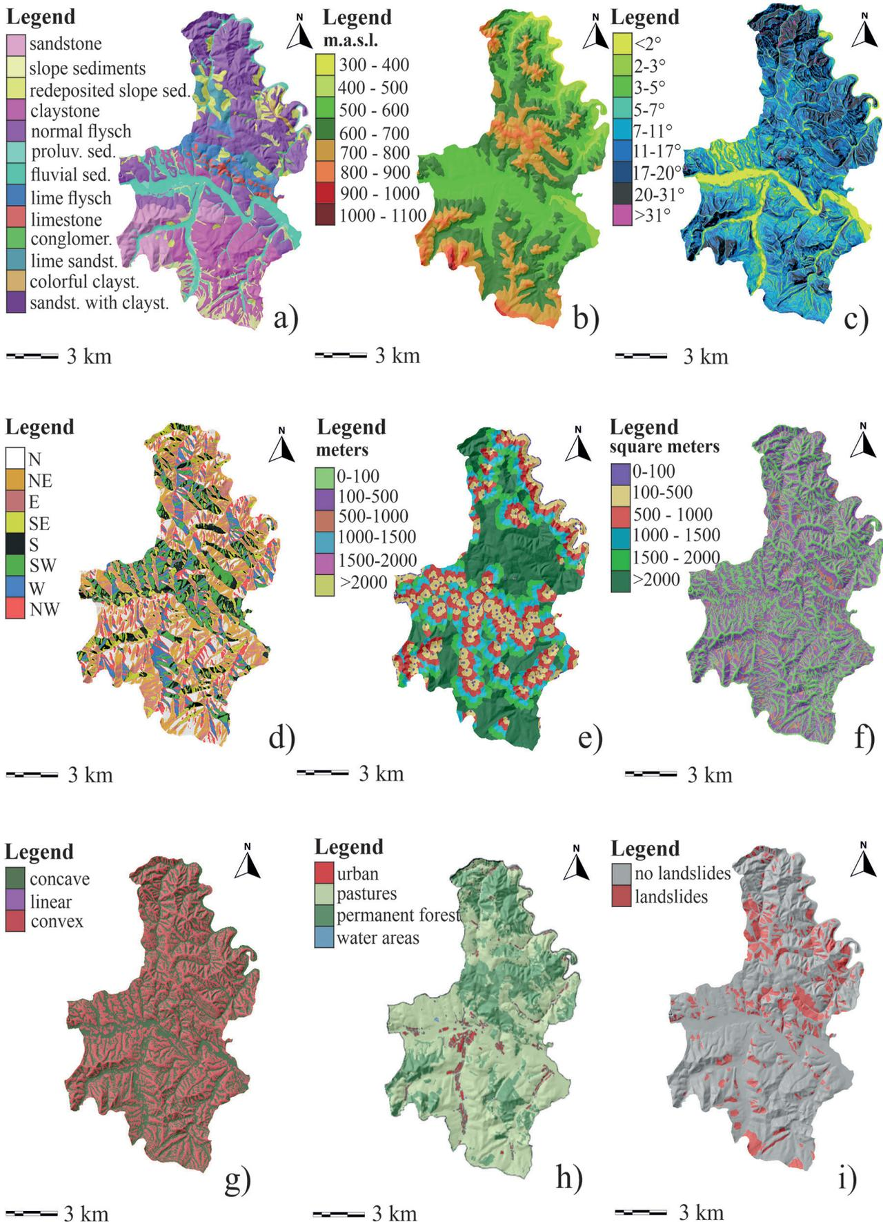
Fig. 2 Parametric maps as they have entered multivariate analysis (a - lithology; b - elevation; c - slope gradient; d - slope orientation; e - slope length; f - contributing areas; g - relief curvature; h - landscape cover; i - slope deformations)
