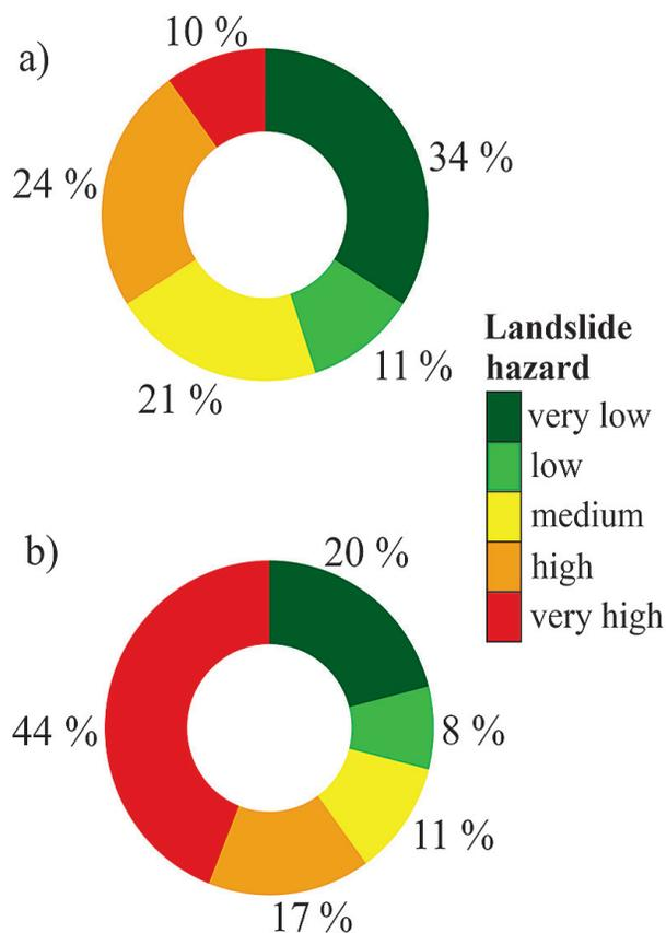
**Fig 4.** Percentage of landslide area that falls within certain landslide hazard levels (a – natural breaks; b – quantile)
